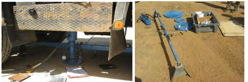
Static Plate Load Test Equipment
